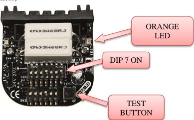
5) Through the TRANSMITTER lens shifts, find the maximum optical alignment based on the Buzzer and LEDs (with high brightness), the increase in the frequency of flashing (until the LEDs is fix on and the whistle of the corresponding BUZZER) indicate a better ALIGNMENT.
