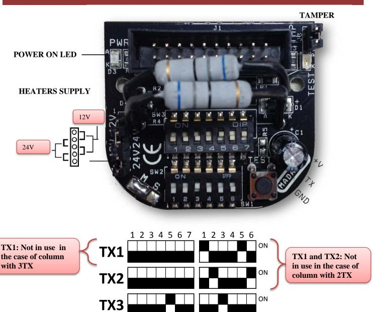
Through DIP 7 in ON (as default) and lighted LED POWER is occur the correct operation of TX optics. The power of the heaters is set by default to 24V; you can use 12V by changing the configuration of the jumper (SW4).
