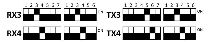
It should be set to ON the DIP on the motherboard RX exclusion 1 + 2
