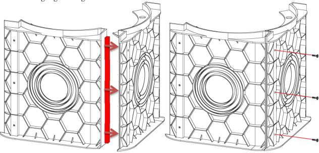
**2.** Insert the third section in the same way and fix with screws.
