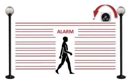
By adjusting the potentiometer counterclockwise to increase the trip time up to 500ms. In this condition ensures that the alarm of a person walking through the barrier, with the advantage of excluding the possibility of any false alarms (ex. animals).
