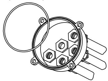
Once the cabling is completed the base cap has to be fixed to the base with relative O-ring.
