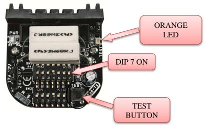
4) Place in the corresponding optical TEST (1 or 2 or 3 or 4) on coral receiver, checking the position of the DIP switch 7 to ON and pressing the dedicated button for 3 seconds until the the BUZZER and the LED TEST turns ON, (with high brightness)
