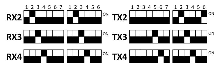
It should be set to ON the DIP on the motherboard RX exclusion 1
