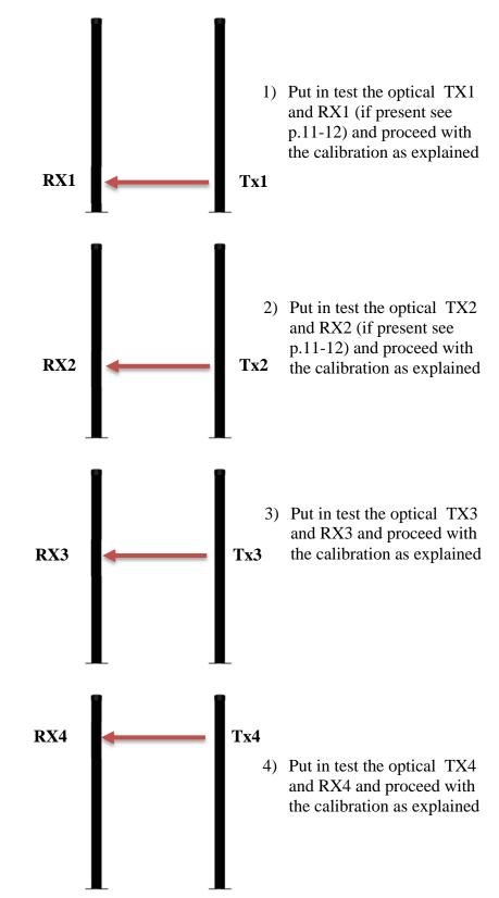
N.B.: during the testing phase of an optical transmitter the other TX not in test are switched off automatically
