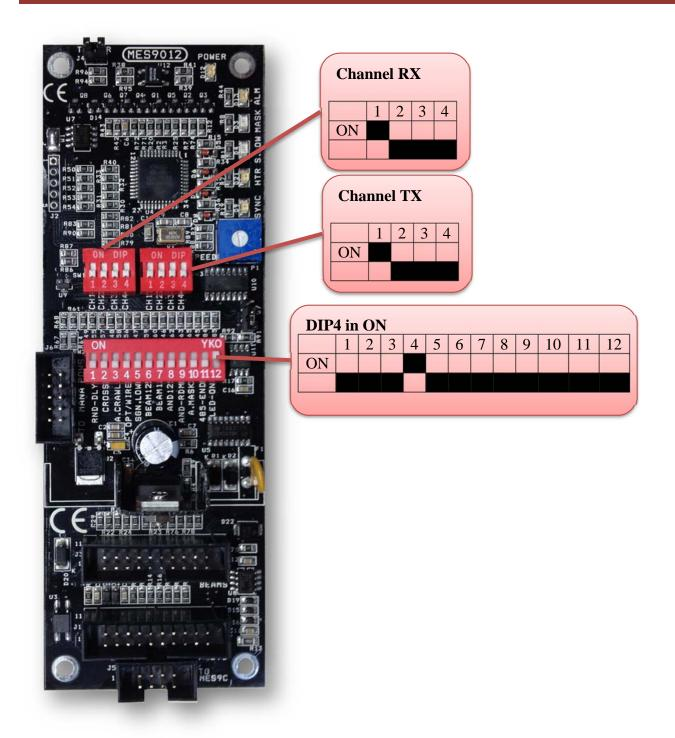
Position in ON DIP 4 on the bench of 12 and select the transmission channel 1 to 3 (default is set to channel 1), on the bench of 4; the selected channel must be the same on both TX and RX boards.
