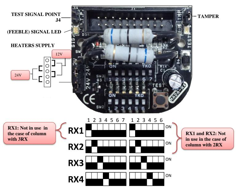
Through DIP 7 in ON (as default) and lighted LED POWER is occur the correct operation of RX optics. The power of the heaters is set by default to 24V; you can use 12V by changing the configuration of the jumper (SW4).
