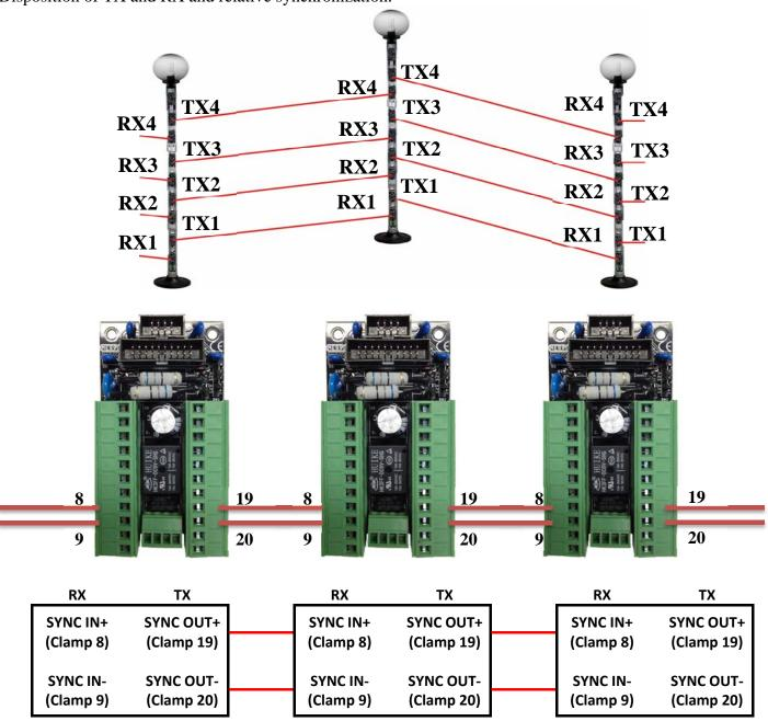
The synchronisms have to be connected according to the diagram above, the  $\mathbf{Sync}$  out corresponds to the TX part of the column and will have to be connected to the  $\mathbf{Sync}$  in on the RX opposite one . You must also connect the negative of power supply in common between the columns; so it is appropriate to use a shielded cable alarm, 2x0, 22, to connect the sync and the screens to negative Vdc of power supply on both columns.
