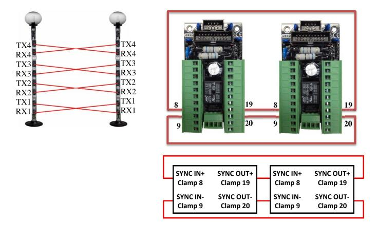
Note: SYNC OUT- and SYNC IN - should not be connected to ground but to the dedicated clamp (terminal numbers are related to the image of p. 11).
