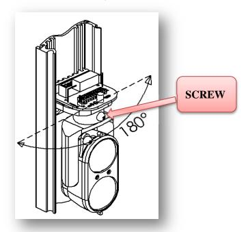
N.B.: FASTEN THE UNLOCKED SCREW AFTER THE ADJUSTMENT
