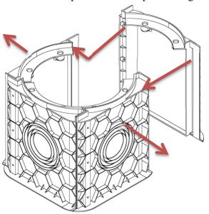
**4.** Insert and well fix the missing screws.
